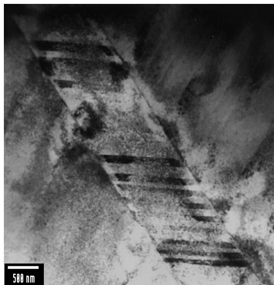
Fig. 3. HP SS316 L, tensile tested at 550 K up to necking. The neutron irradiation dose is 1.5 dpa. Bright field picture shows intersections of different types of twins.
